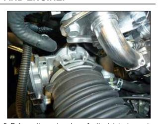
5. Release the spring clamp for the intake hose at the throttle body and then disconnect intake hose from the throttle body.
