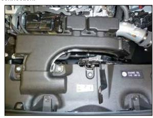
20. Reinstall the fresh air intake duct and secure with the factory hardware.
