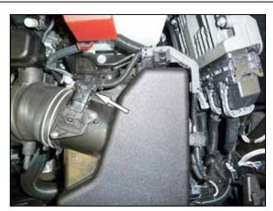
Disconnect the mass air sensor electrical connection.
