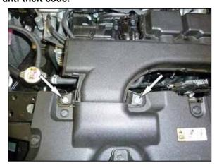
2. Remove the two bolts that secure the fresh air intake duct and then remove the duct from the vehicle.
