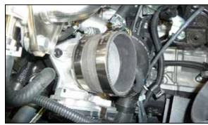
15. Install the provided straight coupler (08711) onto the throttle body and secure with the provided hose clamp.
