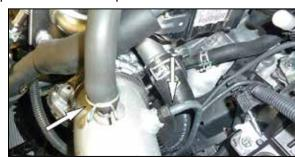
18. Connect the crank case vent line and vacuum line to the vent fittings installed into the K&N<sup>®</sup> intake tube.
