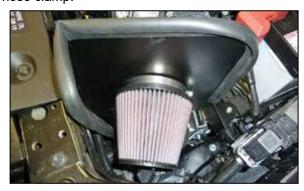
16. Install the K&N® air filter onto the filter adapter and secure with the provided hose clamp.
